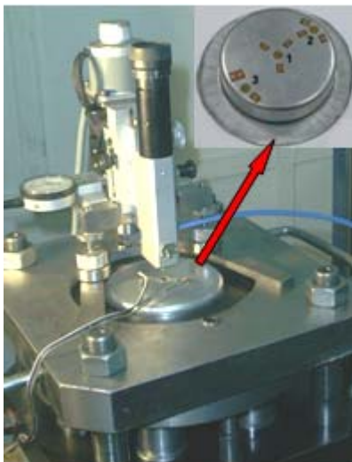
Fig. 2 Drilling a small hole in the center of the bounded strain gauge
